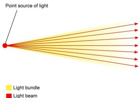
This model is well suited for describing phenomena such as the formation of shadows, reflection, scattering, and refraction of light. At a practical level, ray optics is concerned with the path of light in optical elements such as mirrors, lenses, and prisms and their application in optical devices (microscope, telescope, camera, etc.).
