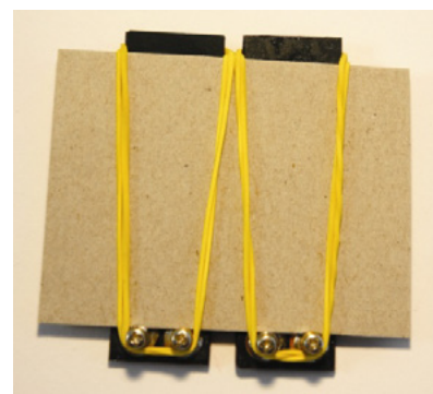
Fig. 6: Mounting the solar cells on a cardboard strip.
