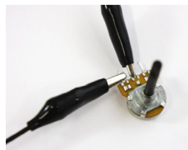
Fig. 17: Connection to a potentiometer via an outside terminal and the middle terminal.
