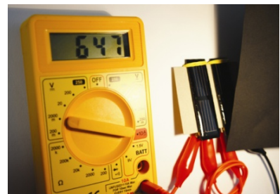
Fig. 13: Partial shading of one of the two solar cells.
