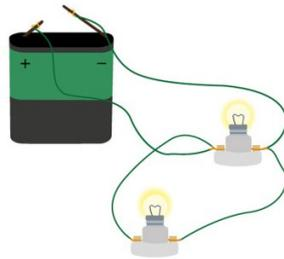
Here the wires are attached in steps from one incandescent lamp to the next.
