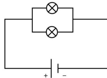
Here the wires are attached at a junction. This variant requires the most cables. The students probably will not figure out this circuit by themselves. That is why the related sketched circuit diagram is explicitly specified again in the observation step and the students are instructed to build this circuit. The students should be capable of recognizing the circuits as being equivalent and graphically converting one to the other.
