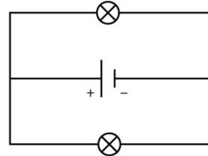
Here, each incandescent lamp is attached directly to the battery terminals. In this case, the underlying concept of “each incandescent lamp has its own electrical circuit” is easier to understand. Most students will probably build this type of circuit.
