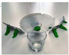
Fig. 1: Experiment setup from behind showing the holders for the mirrors.
