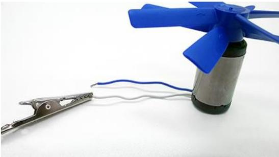
**Note:** The alligator clip must be attached to the exposed wire.
