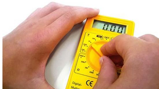
2. Set the digital multimeter to 20 volts.
