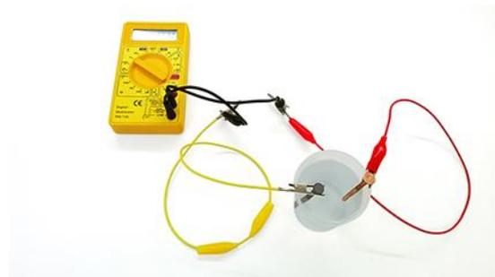
1. Connect the digital multimeter to the two alligator clips in place of the solar motor.
