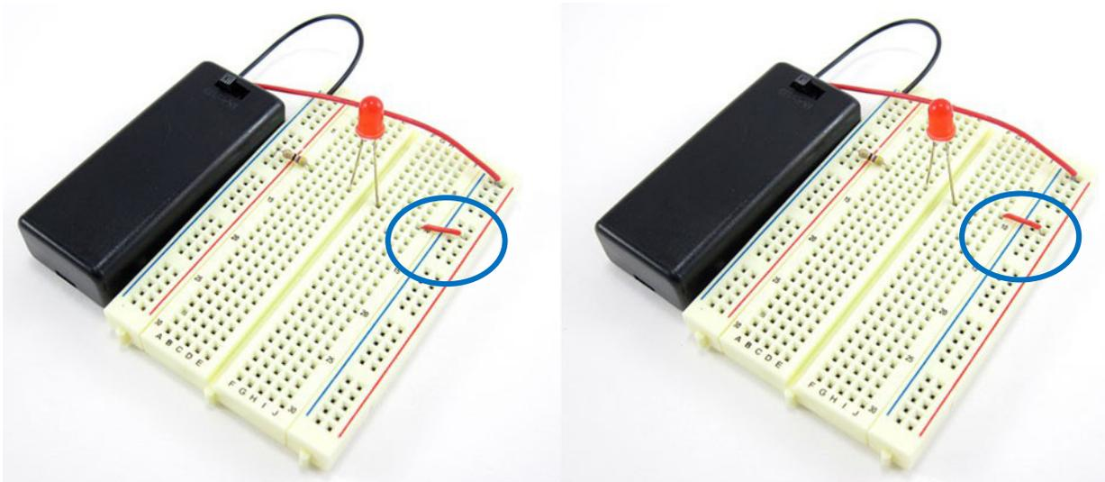
It only takes one misplaced wire or component lead to stop a circuit from working completely. This is why you should always carefully check and double-check your wiring before you test a circuit. If a circuit is not working, double-check the connections and make sure to count the row numbers.
