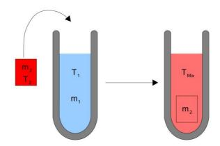
If you now place a solid body into the water, you will notice that the water bath cools down, because a certain amount of the heat is transferred to the solid body in the water bath. As soon as the temperature stops changing, the water and the solid body are in thermal equilibrium. The mixed temperature  $T_{Mix}$  has been reached, and you can calculate the solid's heat capacity by solving the equation (4) for the heat capacity of the cooler substance ( $c_2$ ).
