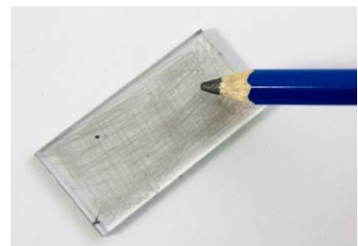
Fig. 3: The conductive side is shaded with graphite using a soft pencil.
