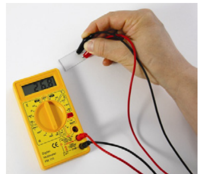
Fig. 2: The conductive side of the clear, transparent glass plate is determined by measuring the resistance.
