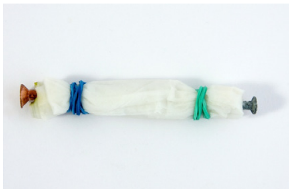
Fig. 10: Completed electrode pack soaked in a solution of table salt.
