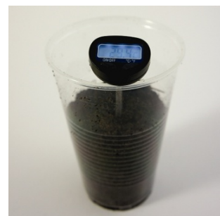
Fig. 3: Temperature measurement inside the cup after exposure to light.
