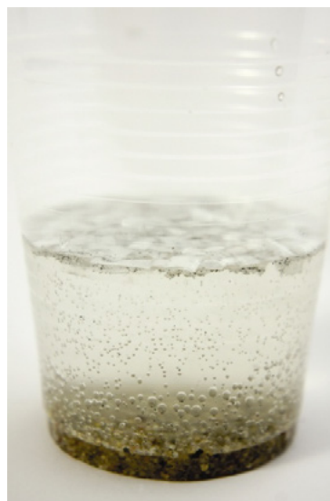
Fig. 2: Our mixture of sand, plastic, water, and salt.
