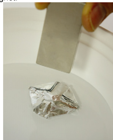
Fig. 4: Move the magnet in circles above the aluminum octagon.
