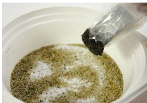
Fig. 1: Using the wrapped magnet to pick up the iron.
