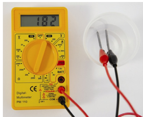
Fig. 3: Measuring the resistance of the aqueous solution.
