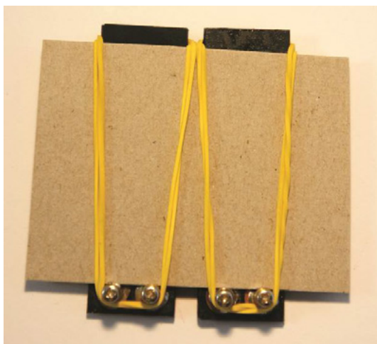
Fig. 10: Mounting the solar cells on a cardboard strip using rubber bands.
