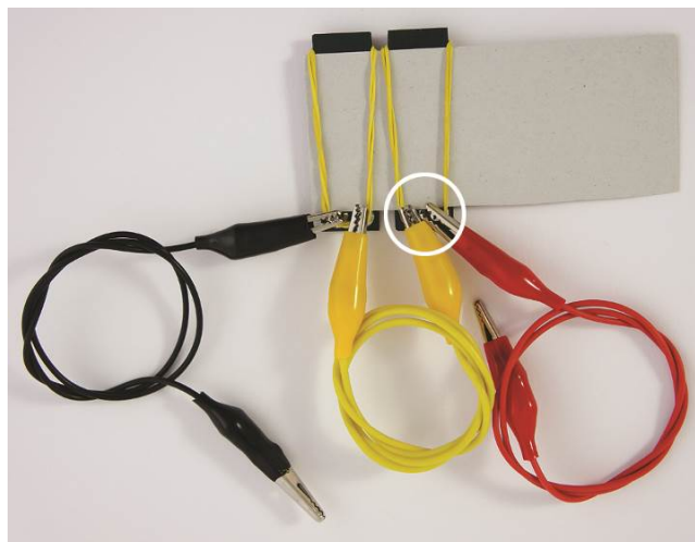
Fig. 9: Make sure that the alligator clips do not touch when you hook them up, or a short circuit will occur.
