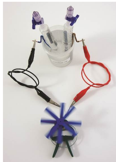
Fig. 7: The cell charged with electrolytic gas can also generate a current.
