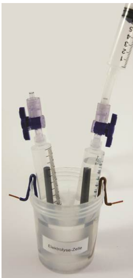
Fig. 5: Suctioning the remaining air; the cylinders fill with soda solution.
