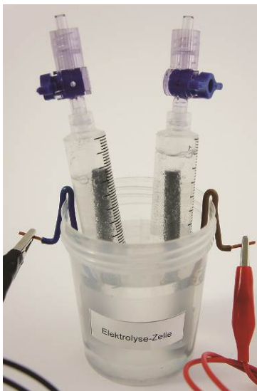
Fig. 6: Generating the gas after attaching the accumulator.
