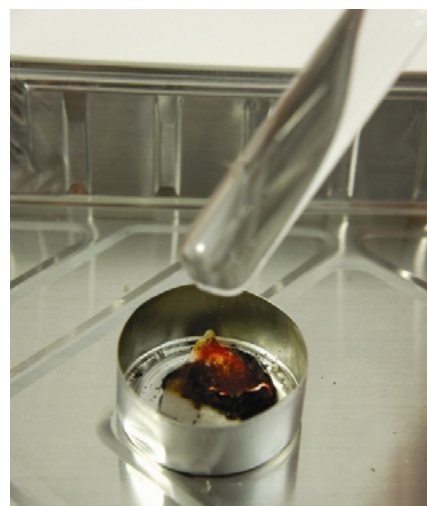
Fig. 3: The cold test tube above the sugar flame.
