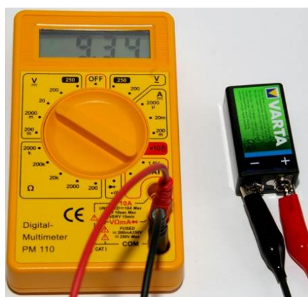
b) Connection of the measuring cables to the digital multimeter and accumulator is correct. A positive voltage is indicated.
