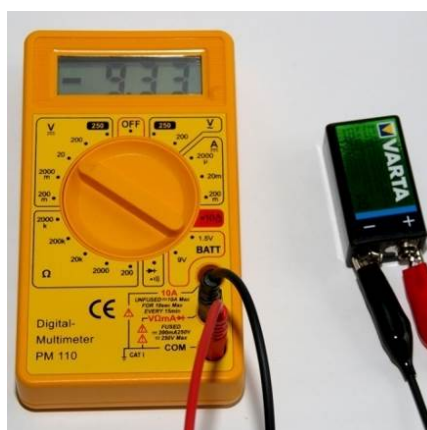
a) Connection of the measuring cables to the digital multimeter is incorrect. A negative voltage is indicated.
