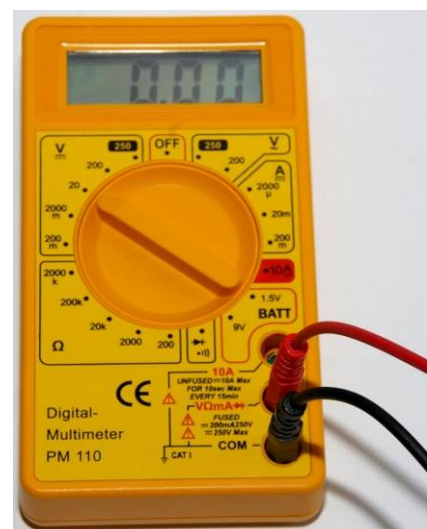
Fig. 4: Correct connection of the measuring cables to the digital multimeter.
