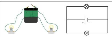
Here, each incandescent lamp is attached directly to the battery terminals. In this case, the underlying concept of "each incandescent lamp has its own electrical circuit" is easier to understand. Most students will probably build this type of circuit.
