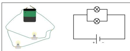
Here the wires are attached at a junction.
