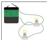
Here the wires are attached in steps from one incandescent lamp to the next.
