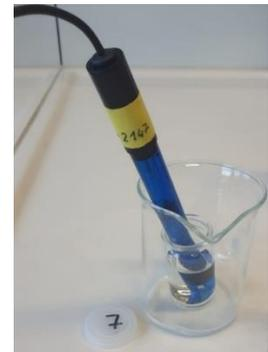
Figure 1: pH electrode in the buffer solution.
